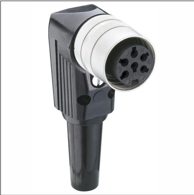
Socket acc. to IEC 61076-2-106, IP40, angular version, with threaded joint, empty housing for reception of crimp contacts, with bend protection, for cable diameter up to 6 mm
